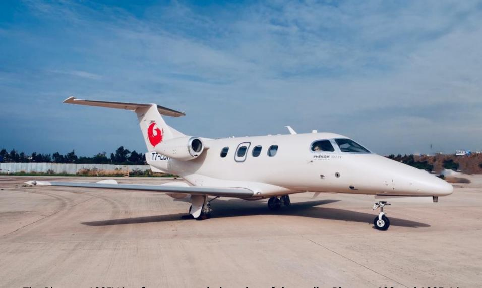
The Phenom 100EV is a faster, upgraded version of the earlier Phenom 100 and 100E. It's Embraer's entry-level airplane, with multifunction spoilers that serve as speed brakes and assist in ground braking, FADEC engine controls, and brake-by-wire systems
